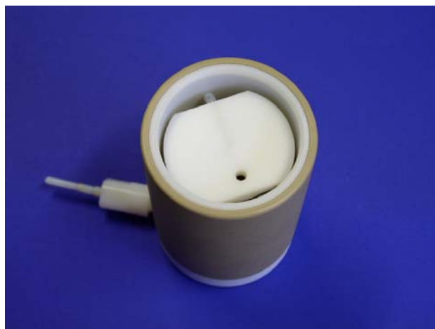
Fig. 7a: Top view after mounting of the reactor outer wall
