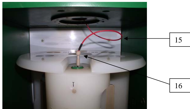
Fig. 13: Insertion of the fiber optic sensor
