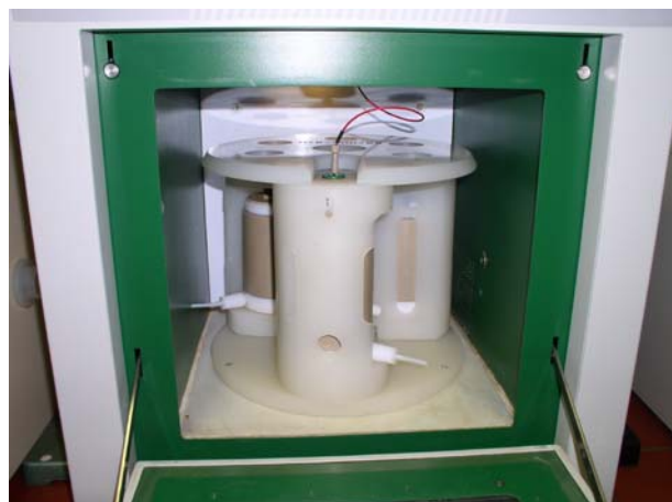
Fig. 14: Hot extraction filtration system HEF 270 inside the microwave system ETHOS 1600 readily prepared to start the extraction
