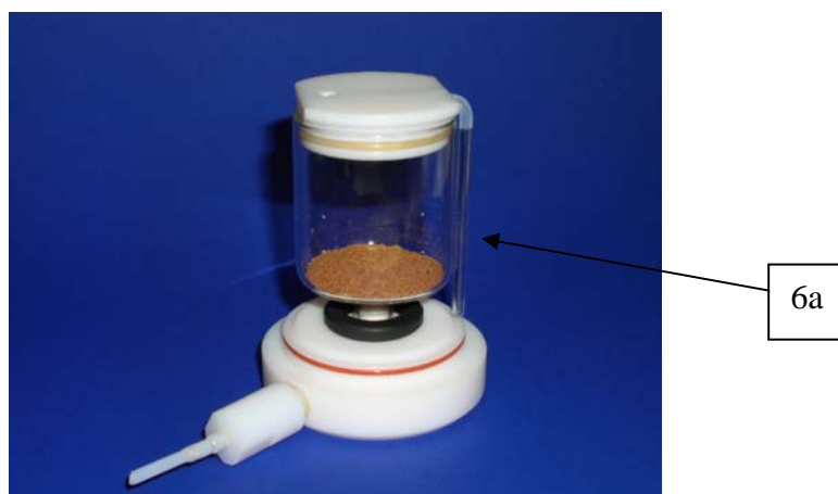
Fig. 6: Mounting of the glass inner vessel with siphon
