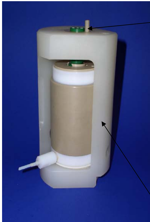
Fig. 9: Reactor inserted into a rotor segment
