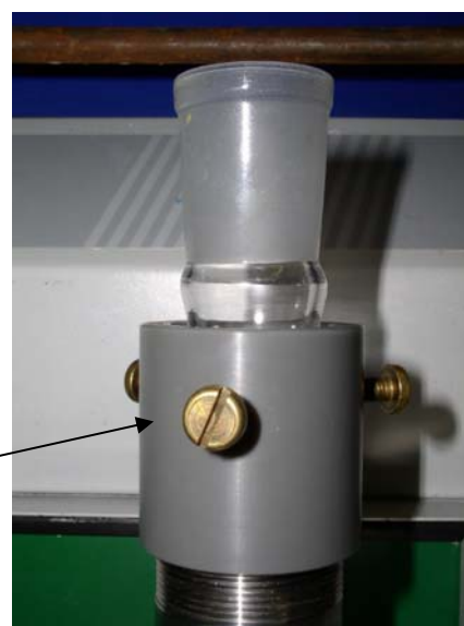
Fig. 3b: Detailed picture of the fixation screws at the top end of the stainless steel tube
