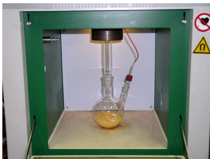
Fig. 1: SRA with 500 mL two-neck flask in microwave system ETHOS MR
