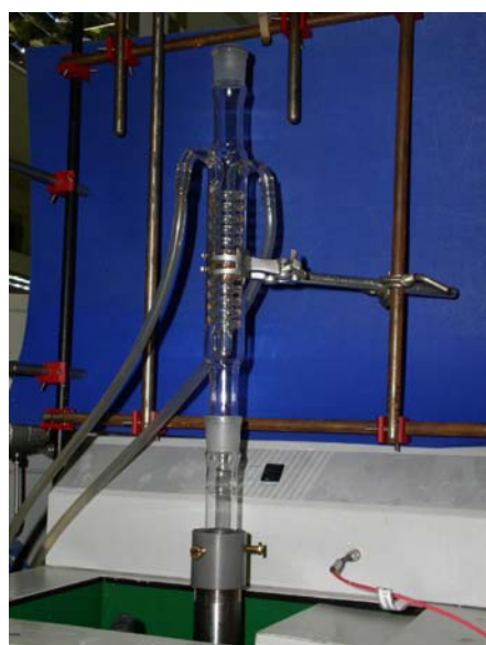
Fig. 5: Mounting of the reflux condenser
