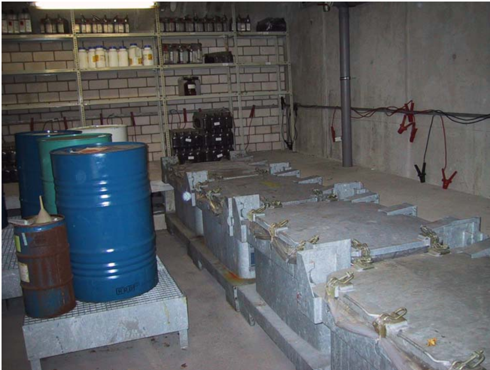
Fig. 2: Picture of closed ASP-containers to store and to transport wastes.
