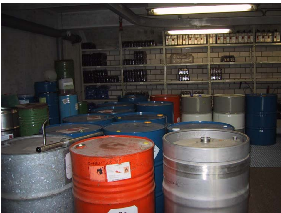
Fig. 1: Picture of an interim store. In front, empty solvent drums are located separately from the chemical wastes stored (at the back).
