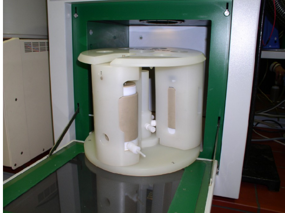
Fig. 12: Mounting the rotor inside the microwave system ETHOS 1600
