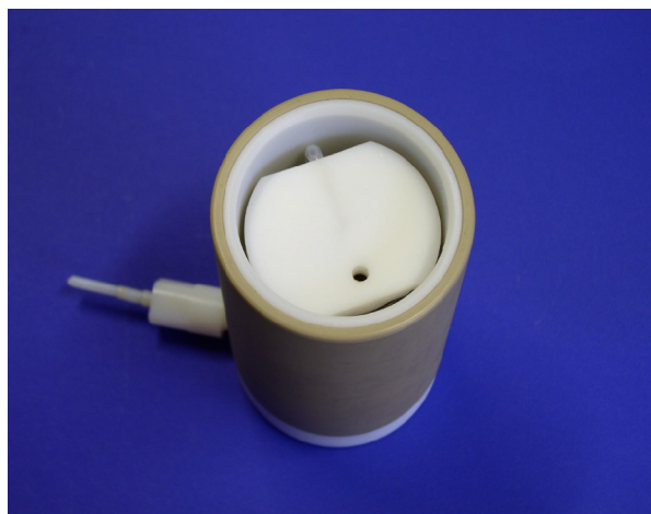
Fig. 7a: Top view after mounting of the reactor outer wall
