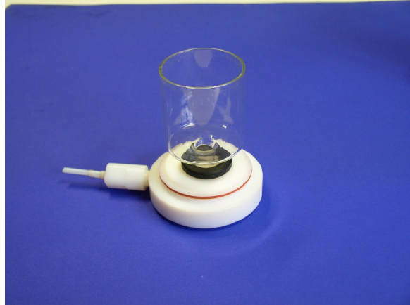
Fig. 3: Inner vessel mounted with Weflon® ring on the base plate
