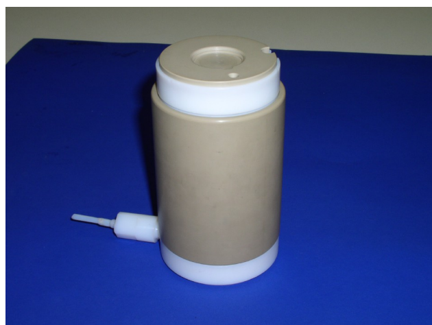
Fig. 8: Completely assembled HEF reactor
