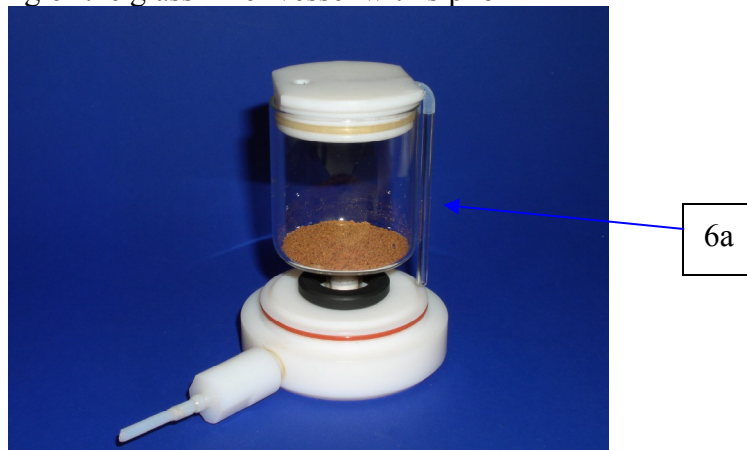
Fig. 6: Mounting of the glass inner vessel with siphon
