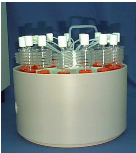
Pic. 3c: 15-segment reflux rotor for group experiments and parallel syntheses
