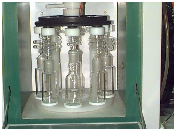
Pic. 3c: 15-segment reflux rotor for group experiments and parallel syntheses
