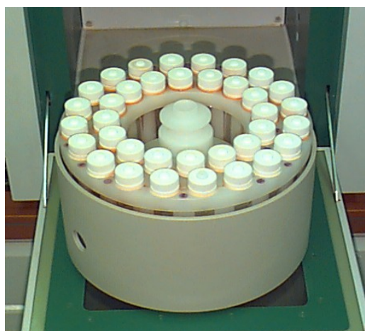
Pic. 4b: 36-segment pressure reactor
