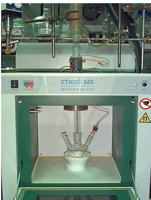
Pic. 2: Microwave system ETHOS MR with reflux apparatus (temperature measurement with fiber optic sensor)
