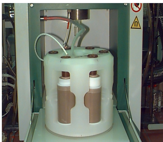
Pic. 4a: 6-segment high-pressure reactor
