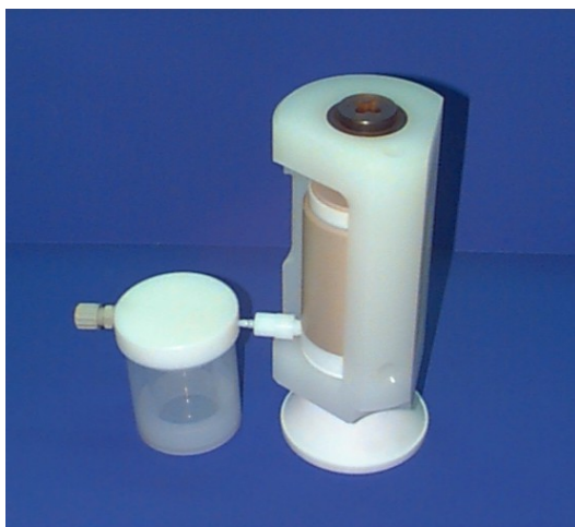
Pic. 5: Hot extraction filtration system
