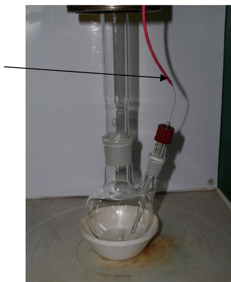
**Fig. 4c:** Threaded pipe with glass protection sleeve
